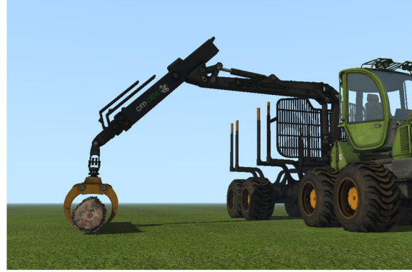
Fig. 9 Model of a log handling crane with two hydraulic actuators
